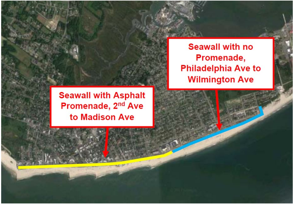
Figure 9: Sections of seawall with and without asphalt promenade.
